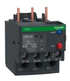
TeSys; TeSys Deca, Thermal overload relay, 690VAC, 0.4 to 0.63A, 1NO+1NC, class 10A, screw clamp
